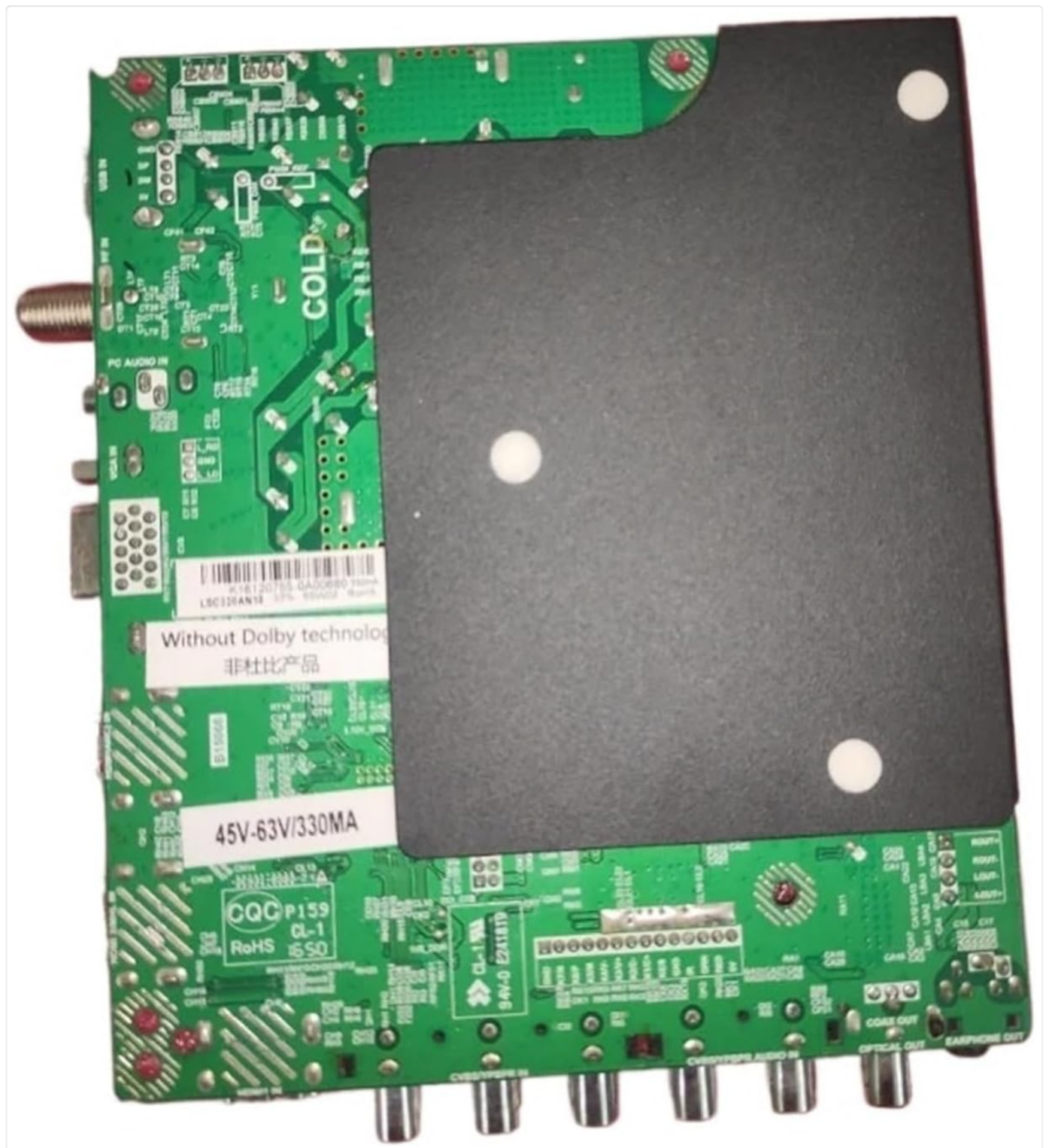
Figure 2: Rear view of the TP.MS3393.PB801 TV Motherboard. This shows the mounting points and the protective cover over sensitive components.
