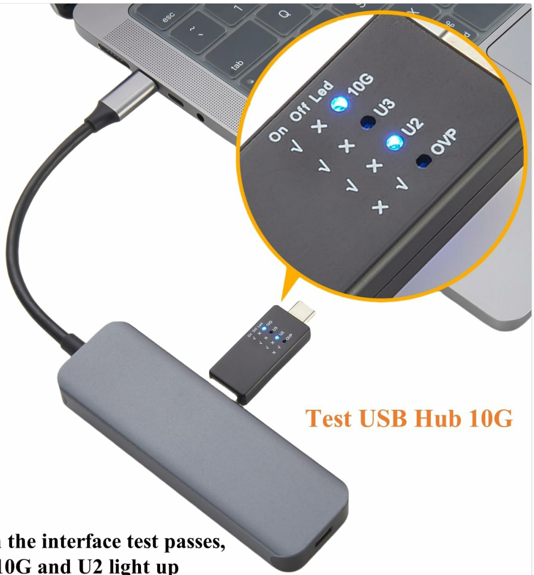
Image 8: Testing a 10G USB hub. The 10G and U2 LEDs are illuminated, confirming the hub's 10Gbps capability.
