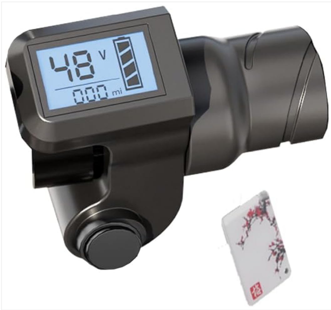
Figure 1: Tomofree Z1/Z2 Electric Bike Throttle with Integrated Display. This image shows the main unit featuring a digital display indicating 48V and 000 miles, a battery level icon, a black control button, and a white key card with a red floral pattern, suggesting an NFC or RFID key function.
