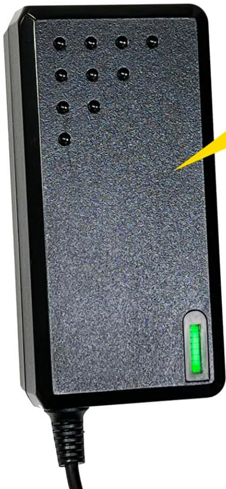
Image 6.1: Diagram illustrating the LED indicator display and its corresponding charging statuses: green flashing for charging, solid green for fully charged, fast red flashing for defective, and fast & slow red flashing for temperature anomaly.
