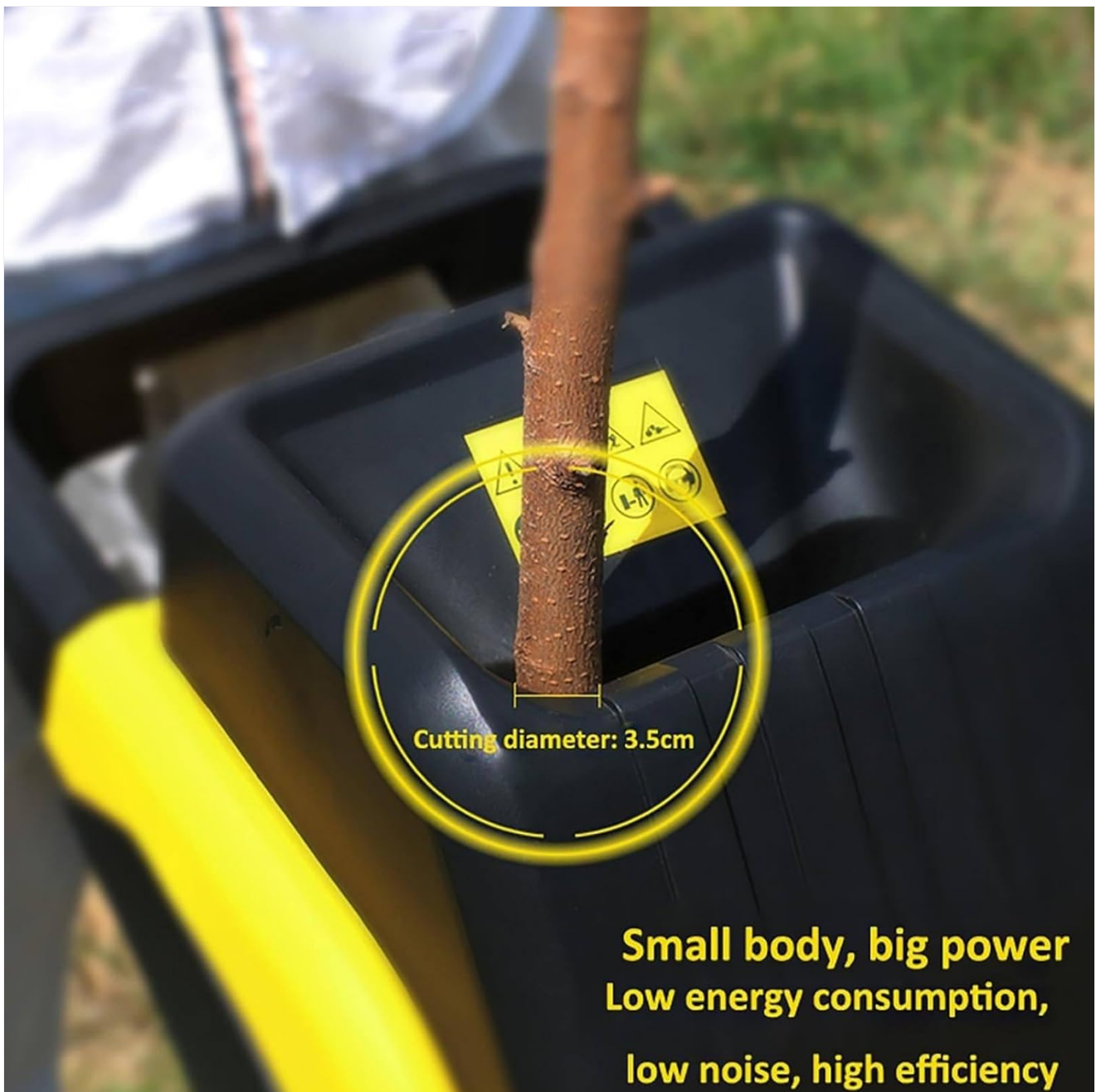
Figure 4.1: Demonstrates feeding a branch into the chipper, illustrating the maximum recommended cutting diameter of 3.5 cm (35mm).
