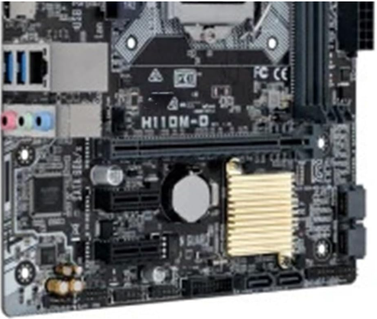
Figure 3.1: Motherboard Rear I/O and Expansion Slots
