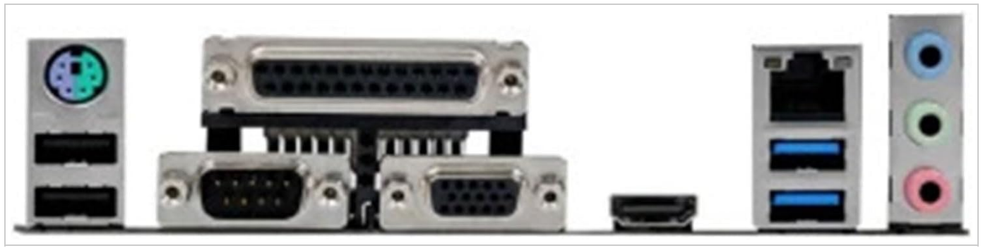
Figure 3.2: Rear I/O Panel Connectors
