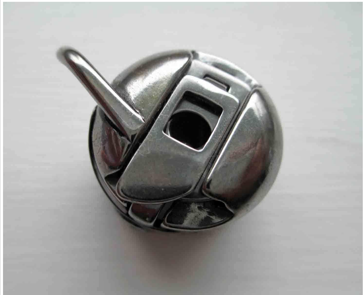
Image 1: Front view of the bobbin case, showing the latch and the opening for the bobbin thread. This view is typical when inserting the bobbin.
