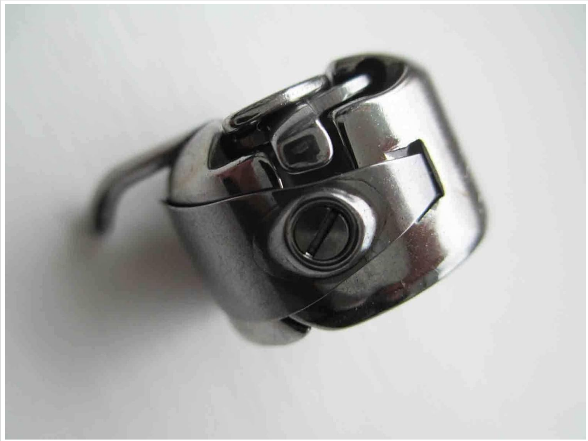
Image 2: Side view of the bobbin case, highlighting the small screw used for adjusting bobbin thread tension.
