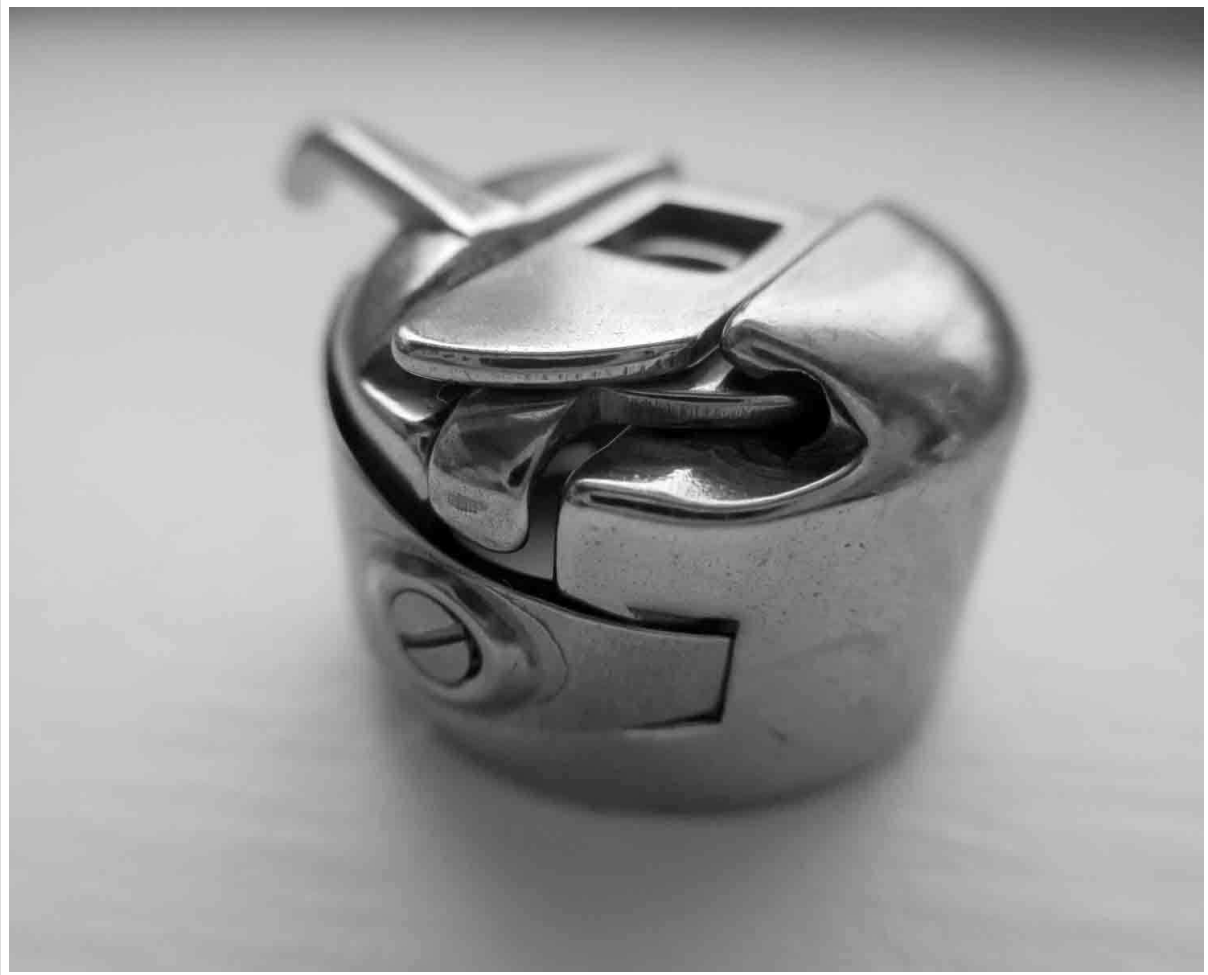
Image 3: An angled view of the bobbin case, providing a clearer perspective of its overall shape and the mechanism for holding the bobbin.
