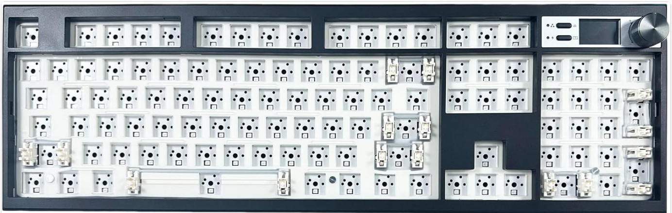
Image: A close-up view of the keyboard's PCB with hot-swappable sockets and pre-lubricated stabilizers, ready for switch installation.
