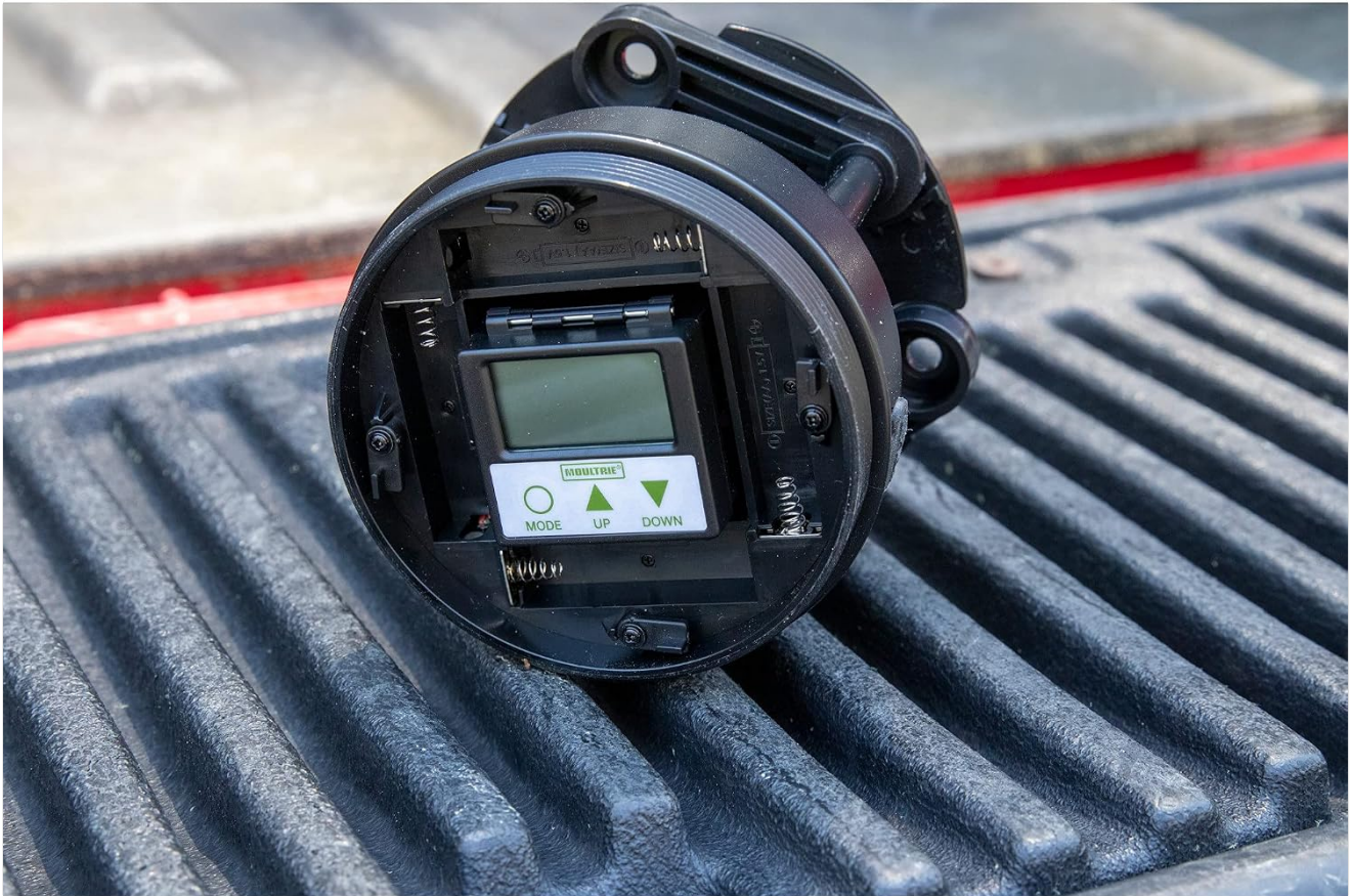
Figure 1: Close-up of the timer's control panel and battery compartment, showing where batteries are inserted.
