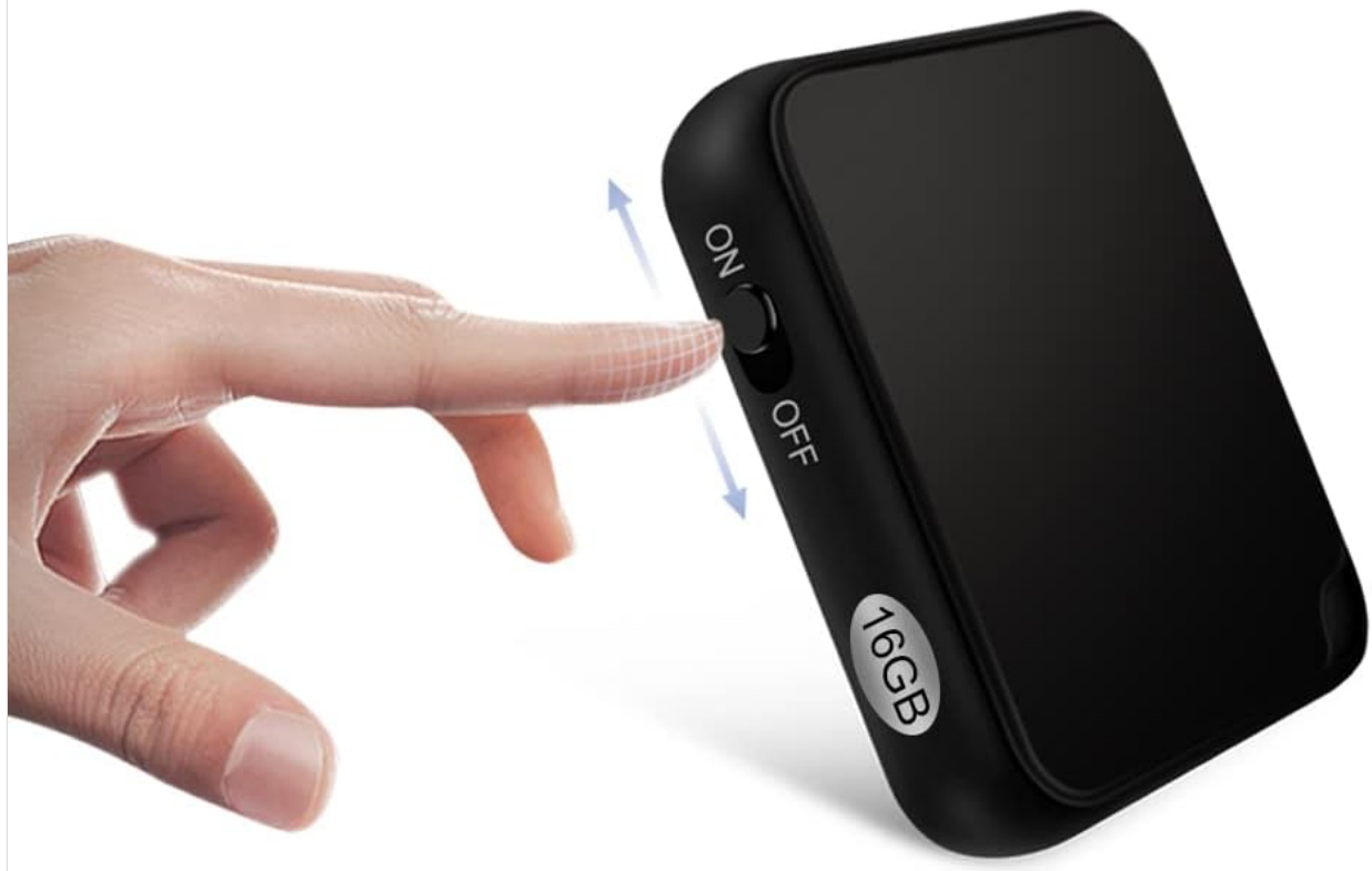
Figure 4: Demonstrating the one-button slide switch for recording and saving.
