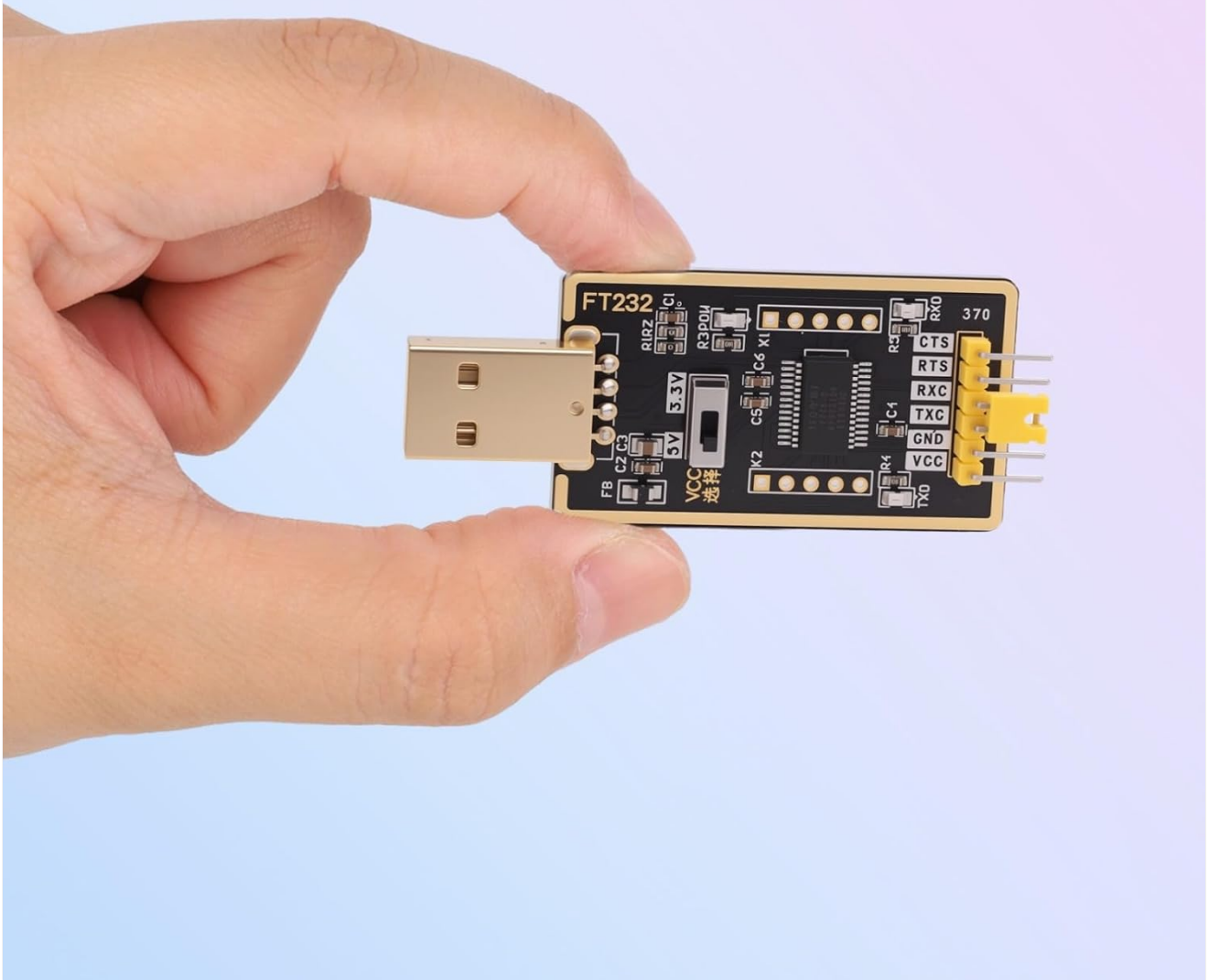
Figure 1: YELUFT USB to TTL Adapter, showing the USB connector and pin headers.
