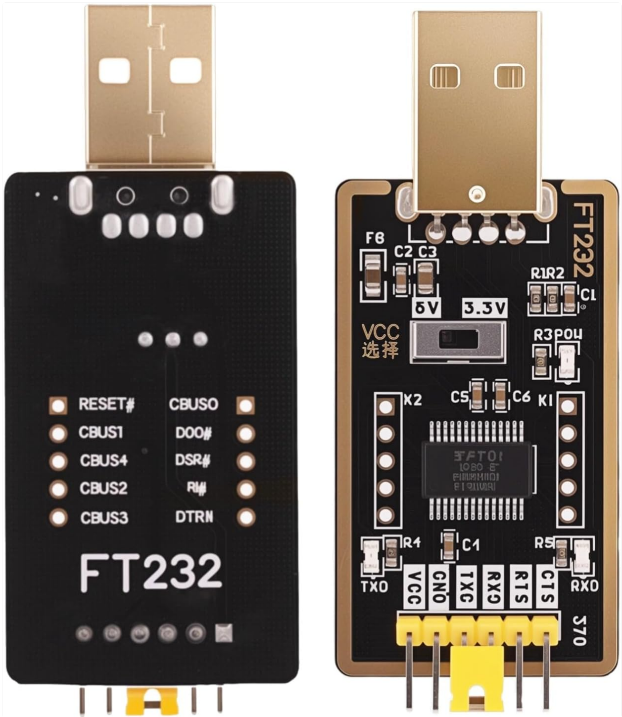
Figure 3: Front and back views of the adapter, showing the voltage selection switch on the front.
