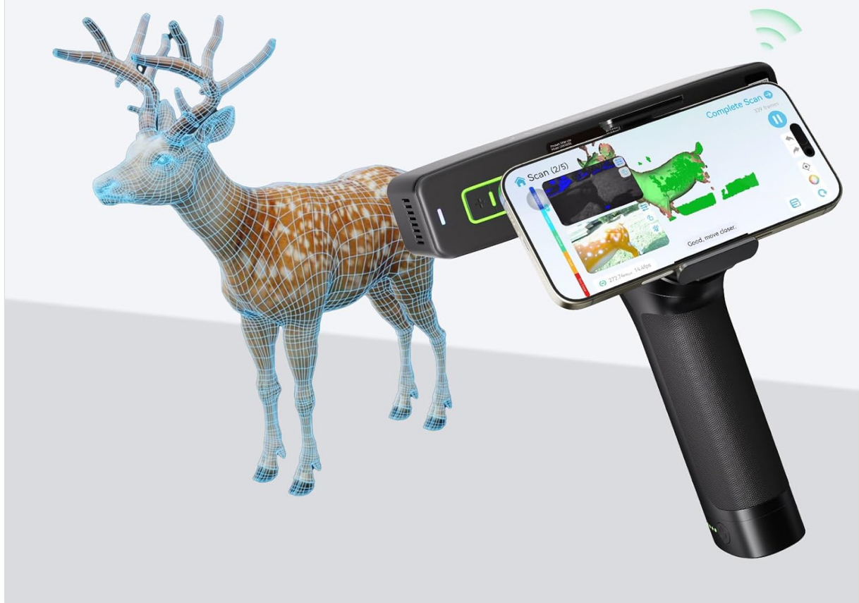
Figure 3.1: Real-time mobile preview of a 3D scan, showing the object being digitized on a smartphone screen, with the Creality-branded scanner.
