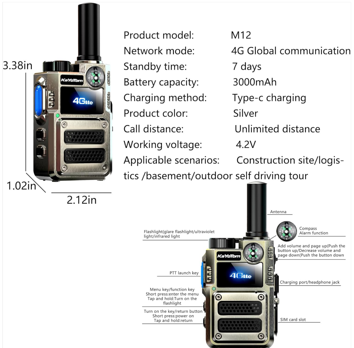
Figure 5: KAYOTOM M12 radio with labeled dimensions and key features.
