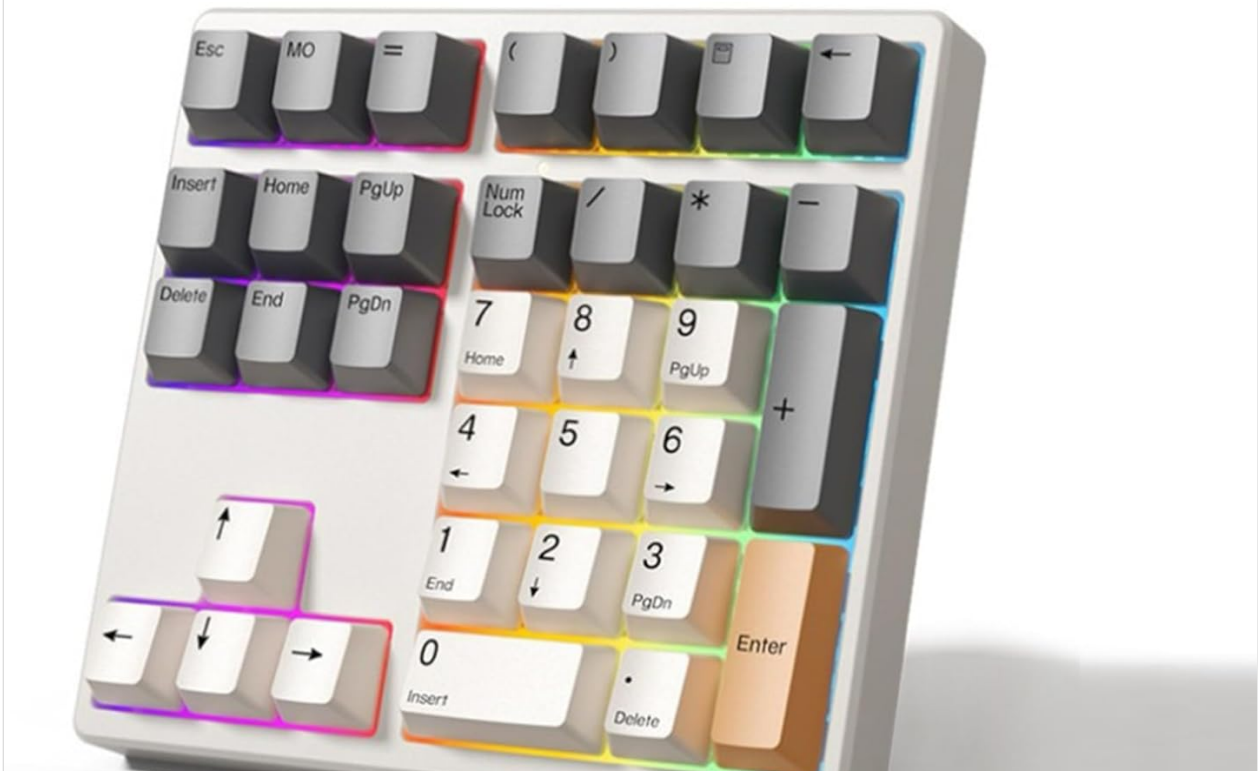
Image: Overview of the 34-key mechanical numeric keypad, highlighting its comprehensive layout including numeric, arrow, and function keys.
