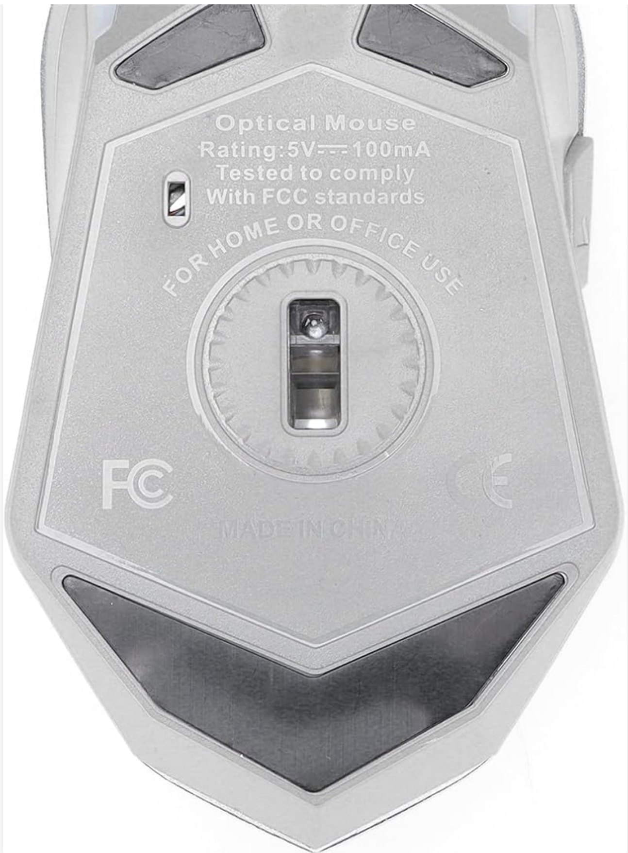
Figure 4: Underside of the Haofy Gaming Mouse. This image highlights the optical sensor opening and the glide pads, along with product information.
