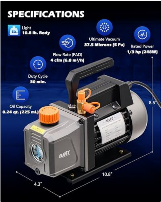
Image 4.1: Visual representation of the vacuum pump's key specifications and dimensions.
