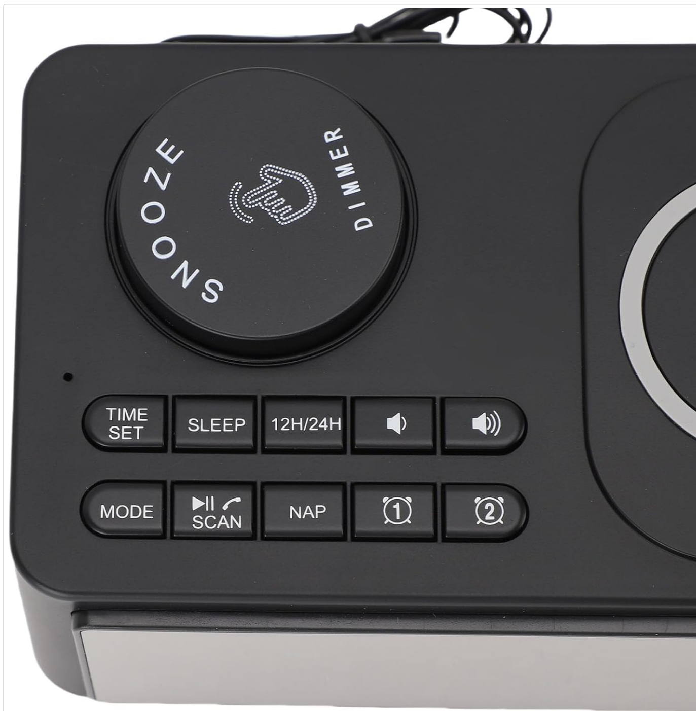
Image 4.1: Detailed view of the control buttons including TIME SET, SLEEP, 12H/24H, volume controls, MODE, PLAY/SCAN, NAP, and alarm buttons (1 and 2).
