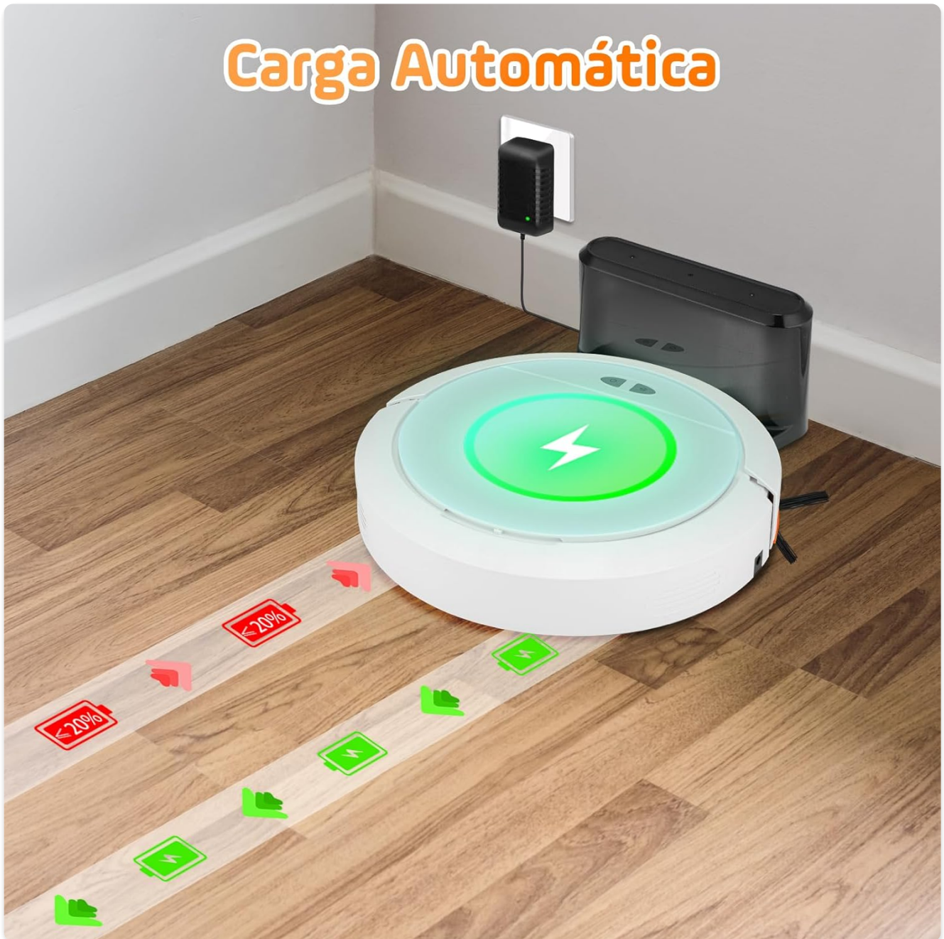
Figure 4.1: The robot automatically returns to its charging base when battery is low or cleaning is complete.
