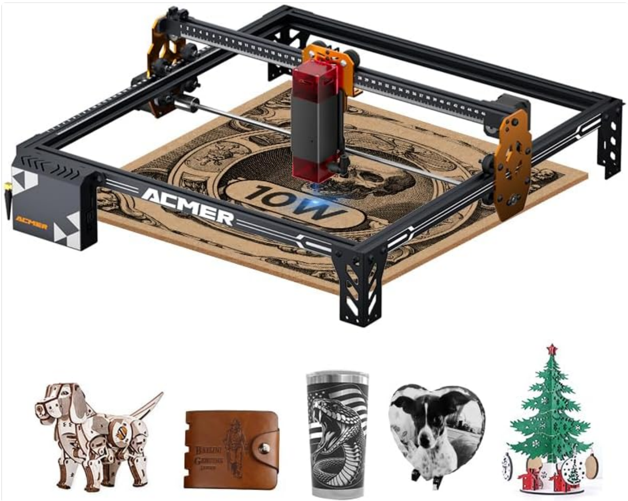
Figure 3.1: The ACMER P1 S Pro 10W Laser Engraver, showcasing its open-frame design and examples of engraved items such as a wooden dog, leather wallet, and metal tumbler.
