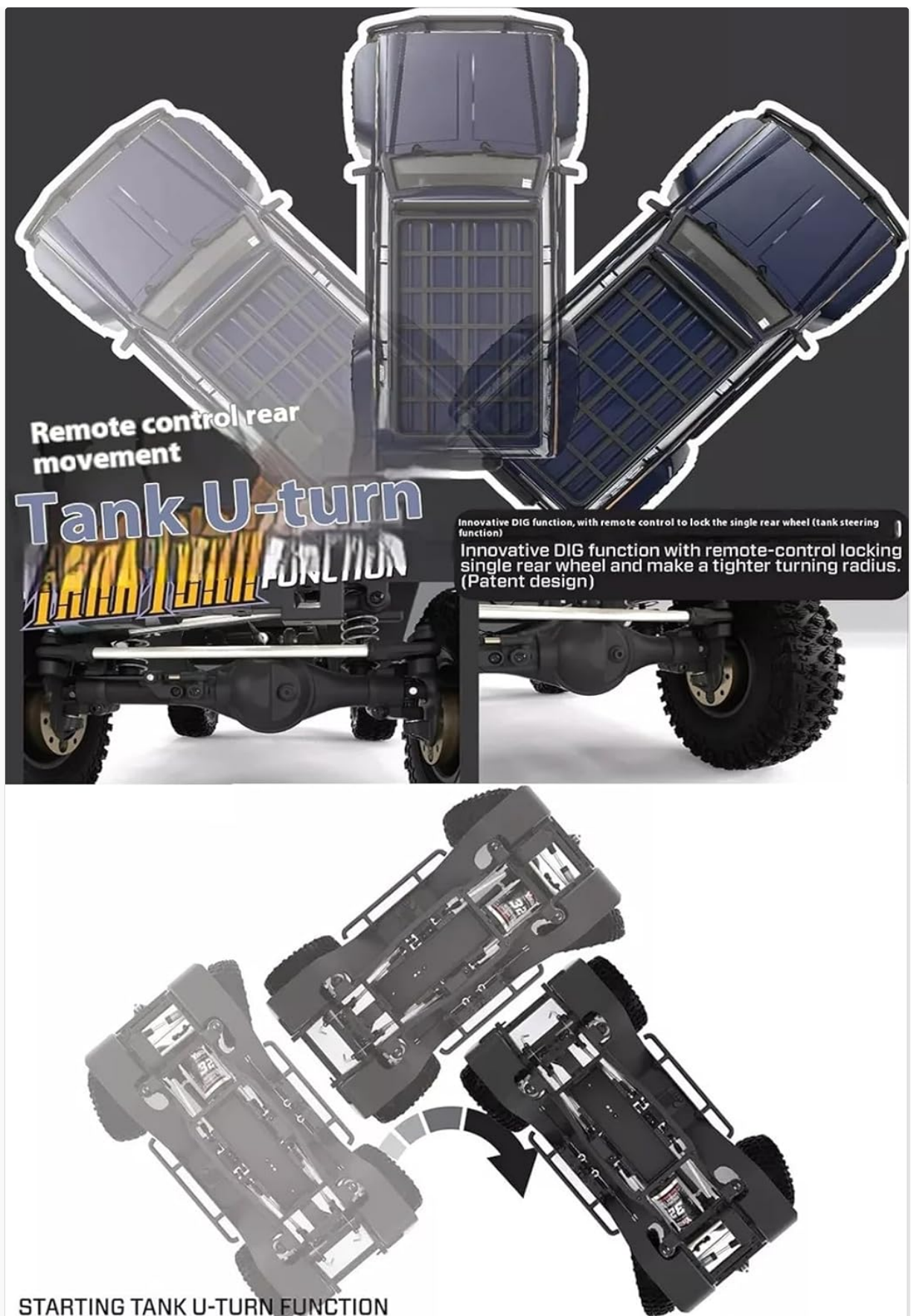
Figure 4: Visual explanation of the Tank U-turn function, showing remote control input and vehicle movement.
