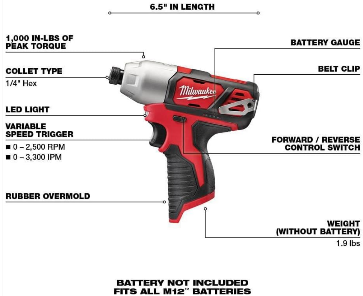
Figure 1: Labeled diagram of the Milwaukee M12 1/4-inch Hex Impact Driver, highlighting key features such as the 1/4" Hex Collet Type, LED Light, Variable Speed Trigger, Rubber Overmold, Battery Gauge, Belt Clip, and Forward/Reverse Control Switch. The diagram also indicates the tool's length (6.5 inches) and weight without battery (1.9 lbs).
