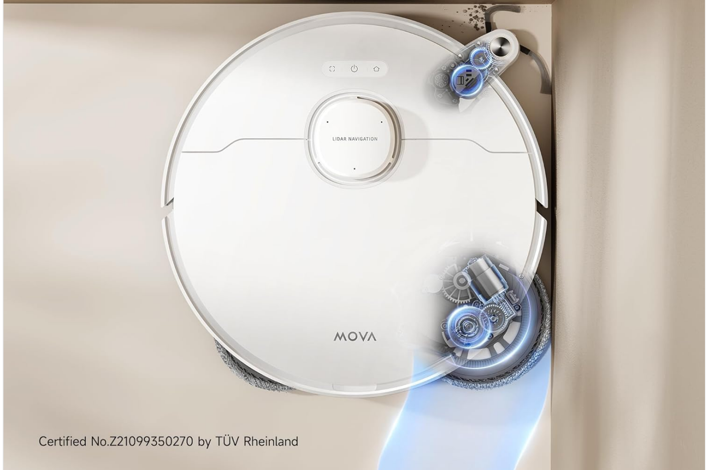
Figure 6: The Dual Flex Arm design allows the robot to extend its side brush and mop, ensuring thorough cleaning in corners and along edges.
