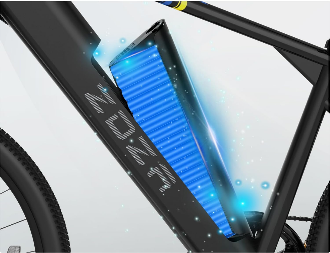
Image: Close-up of the 375Wh rechargeable and removable lithium battery, highlighting its capacity and anti-theft lockable design.
