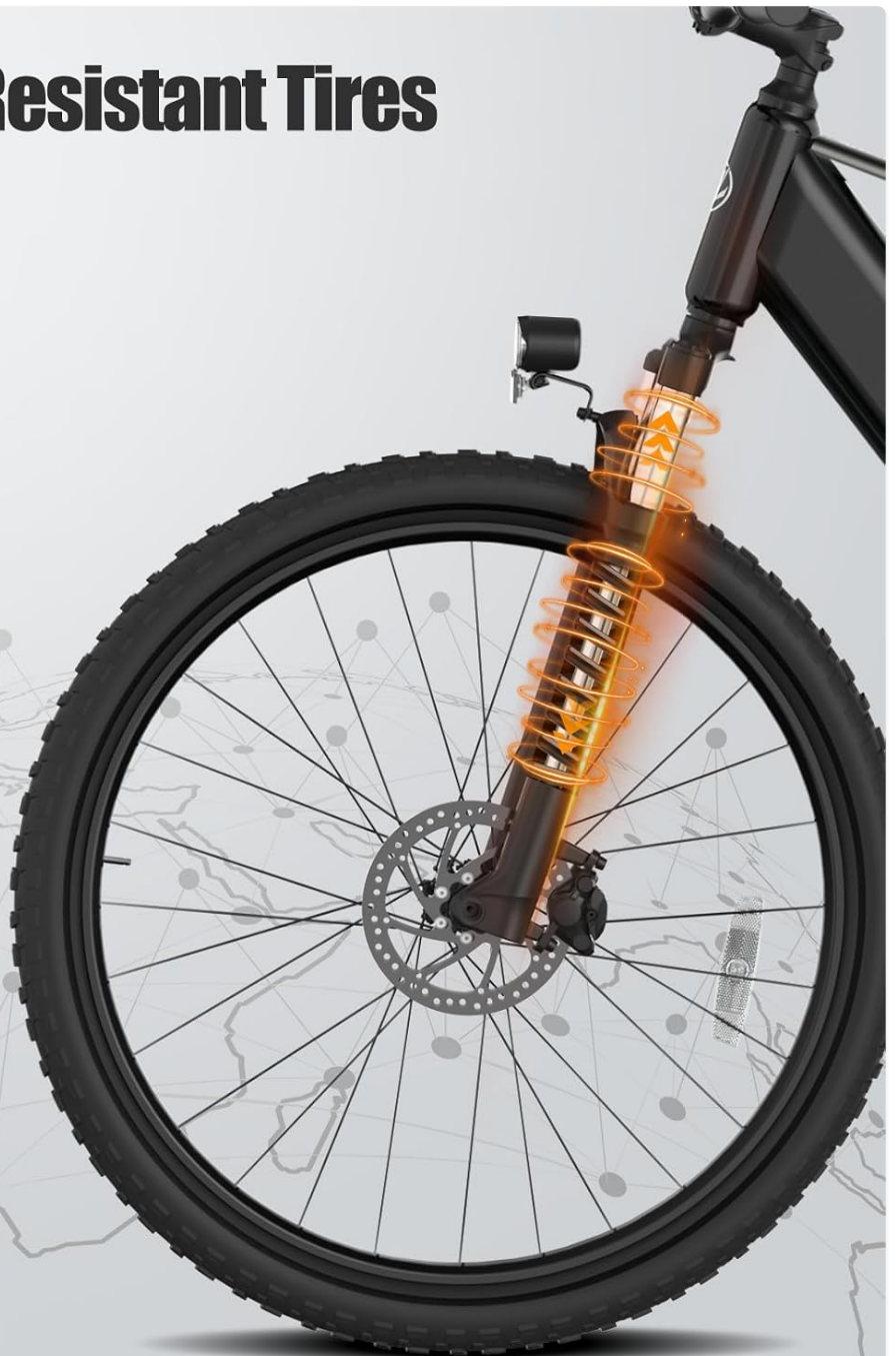
Image: Close-up of the 26-inch puncture-resistant tires and front suspension, highlighting suitability for various terrains.
