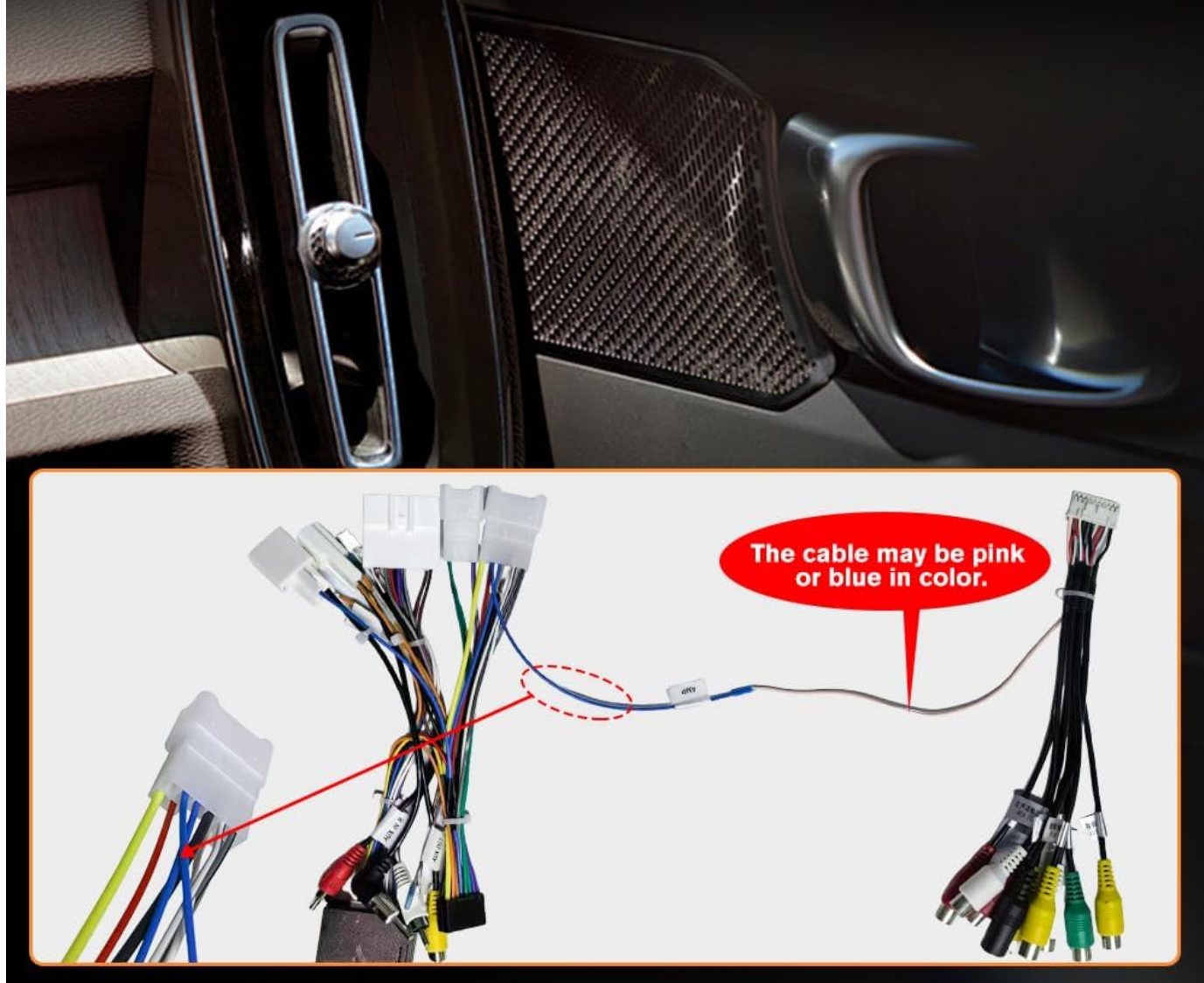
Image: Specific wiring detail for Harman Kardon systems, showing the AMP wire connection.
