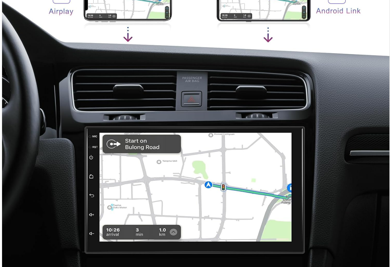
Figure 5.3: Illustration of Mirror Link displaying smartphone content on the car stereo screen.
