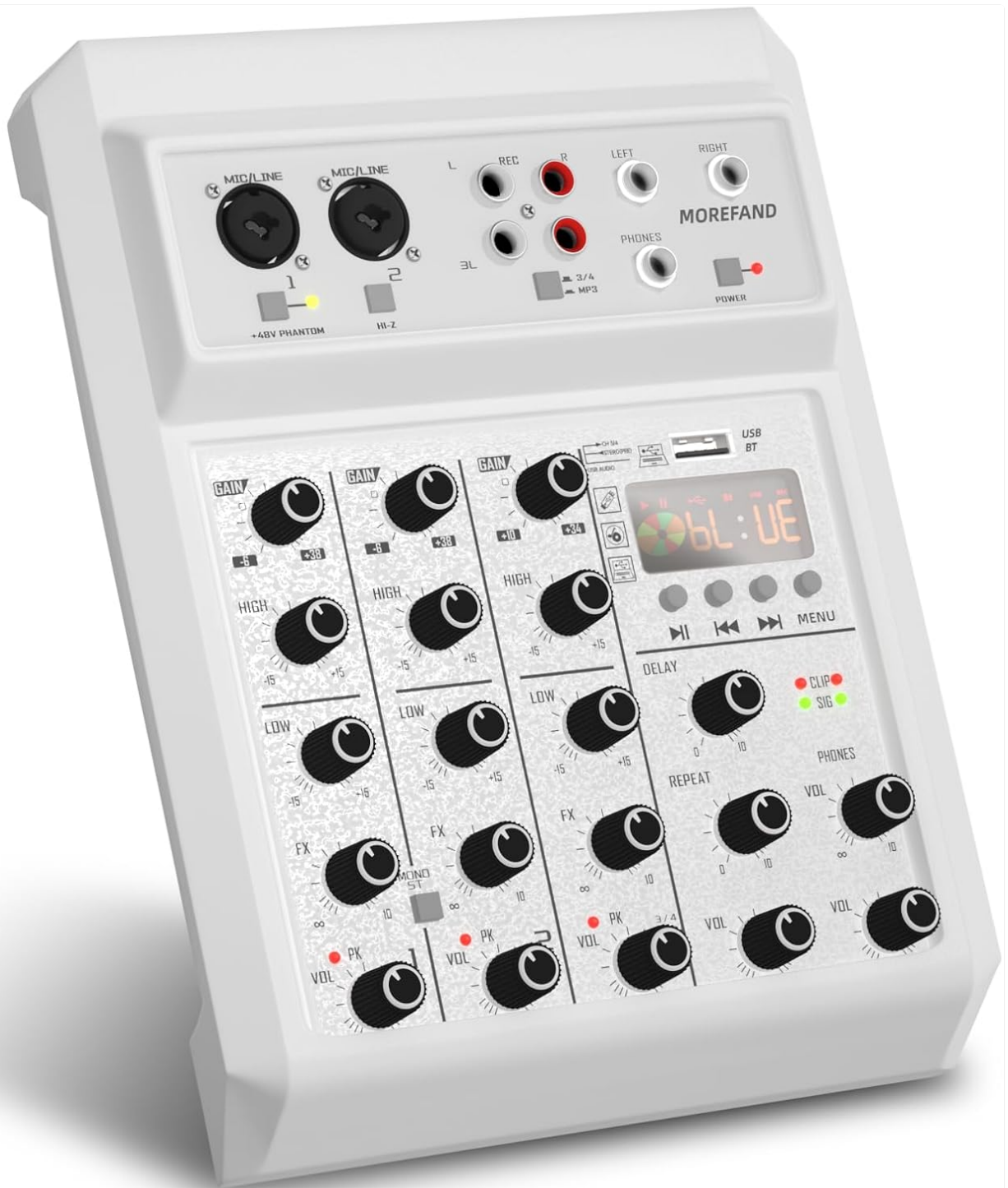
Image: Front view of the MOREFAND RE-405 audio mixer, highlighting its compact design and control layout.
