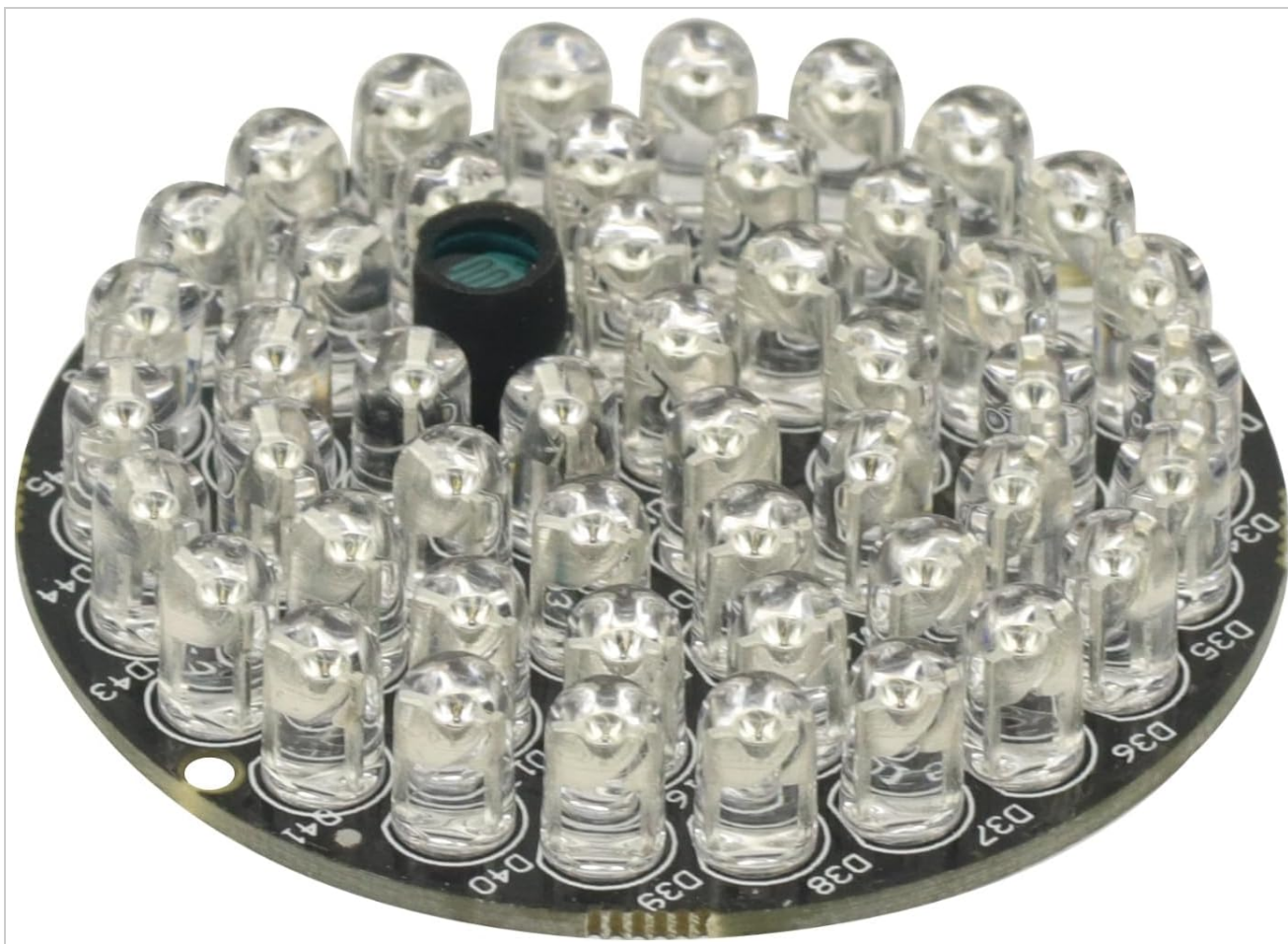
Figure 2: Front view of the 48-LED IR Illuminator board, featuring 48 individual F5 LEDs and a central photocell for automatic operation.
