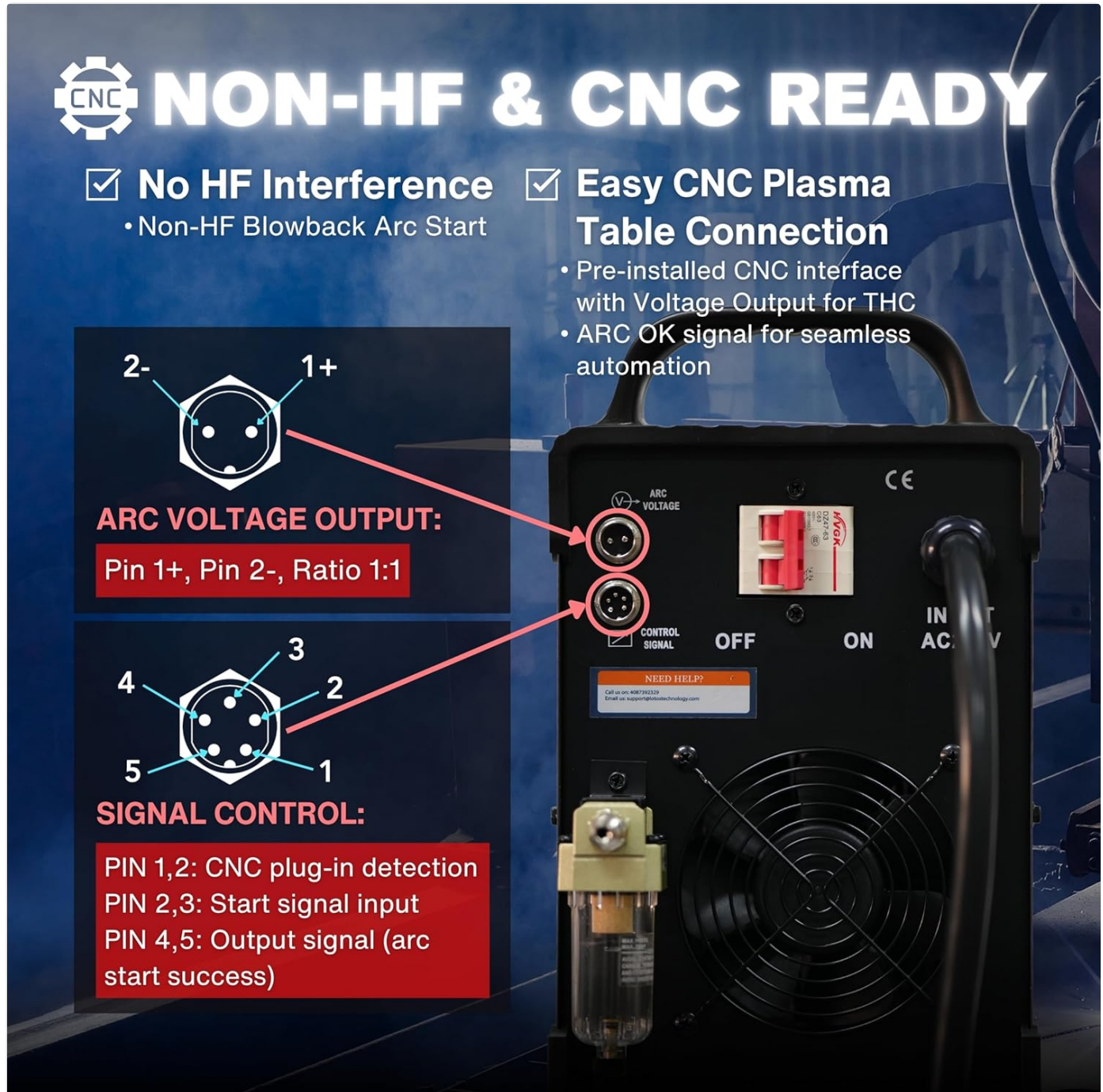
Image: A detailed view of the rear panel of the plasma cutter, highlighting the ARC VOLTAGE OUTPUT (2-pin) and SIGNAL CONTROL (5-pin) ports for CNC integration.
