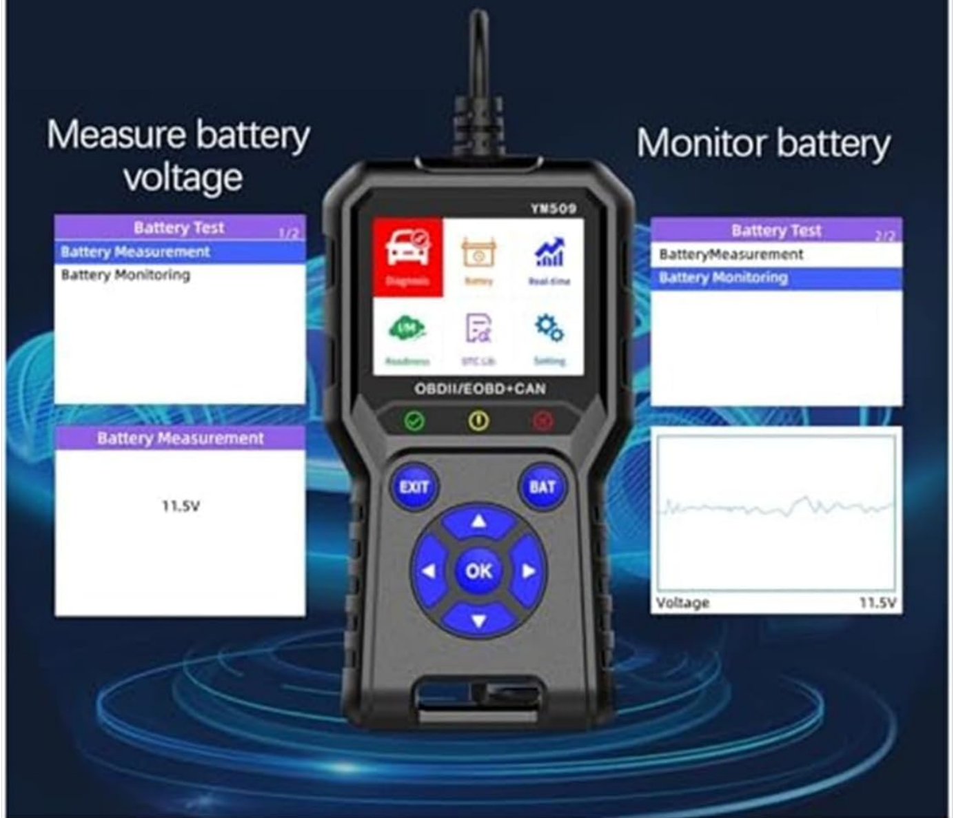
Image 3.4: The YM509's battery monitoring interface. It shows both a static voltage measurement (e.g., 11.5V) and a real-time graph illustrating battery voltage fluctuations, providing a comprehensive view of battery status.
