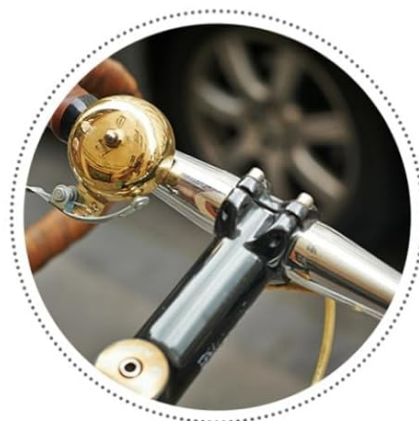
Image 4.1: Detailed view of the bell's mounting clamp and the screw used for attachment, along with the ringing lever.
