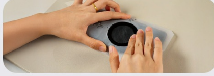
Image: Steps for attaching a magnetic ring to a non-MagSafe phone.
