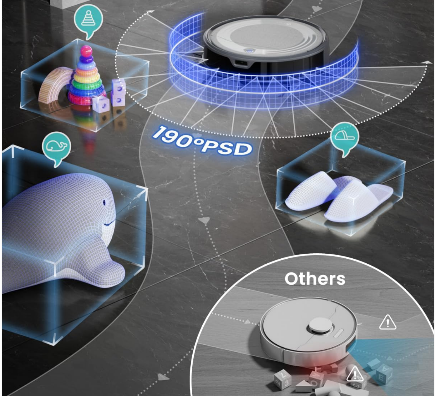
Figure 8: A visual explanation of the Lefant M310 Ultra's precision obstacle recognition and evasion capabilities. It highlights the 190-degree PSD (Position Sensitive Detector) technology that allows the robot to detect and avoid various objects like toys and slippers, preventing collisions and ensuring smooth navigation.
