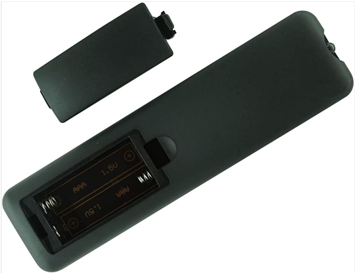
Figure 2: Battery compartment open, illustrating battery placement.
