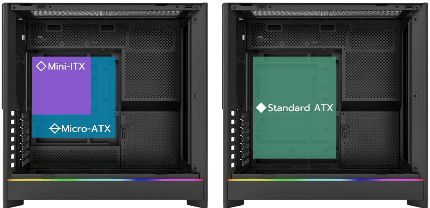
Image 8.1: Visual representation of motherboard form factor compatibility within the case, indicating supported sizes.
