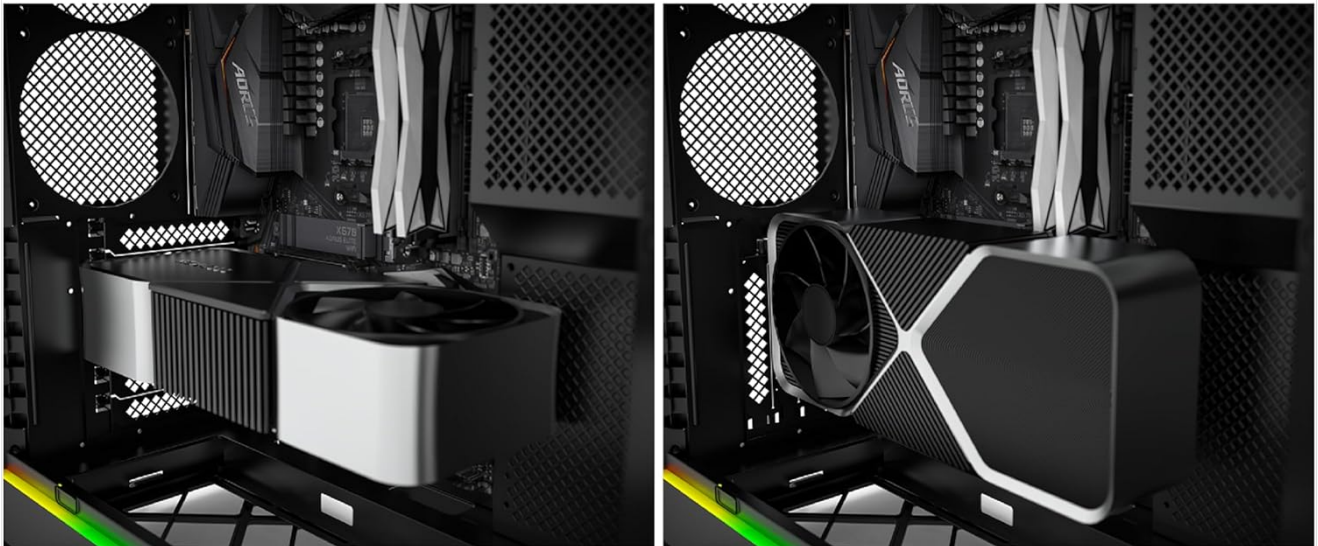
Figure 3.5: Comparison showing horizontal and vertical GPU mounting options using the rotatable PCIe slots.
