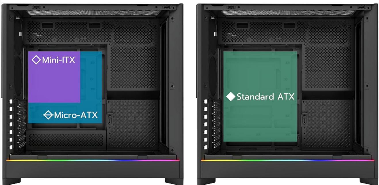
Figure 3.2: Diagram illustrating motherboard compatibility for Mini-ITX, Micro-ATX, and Standard ATX sizes within the case.
