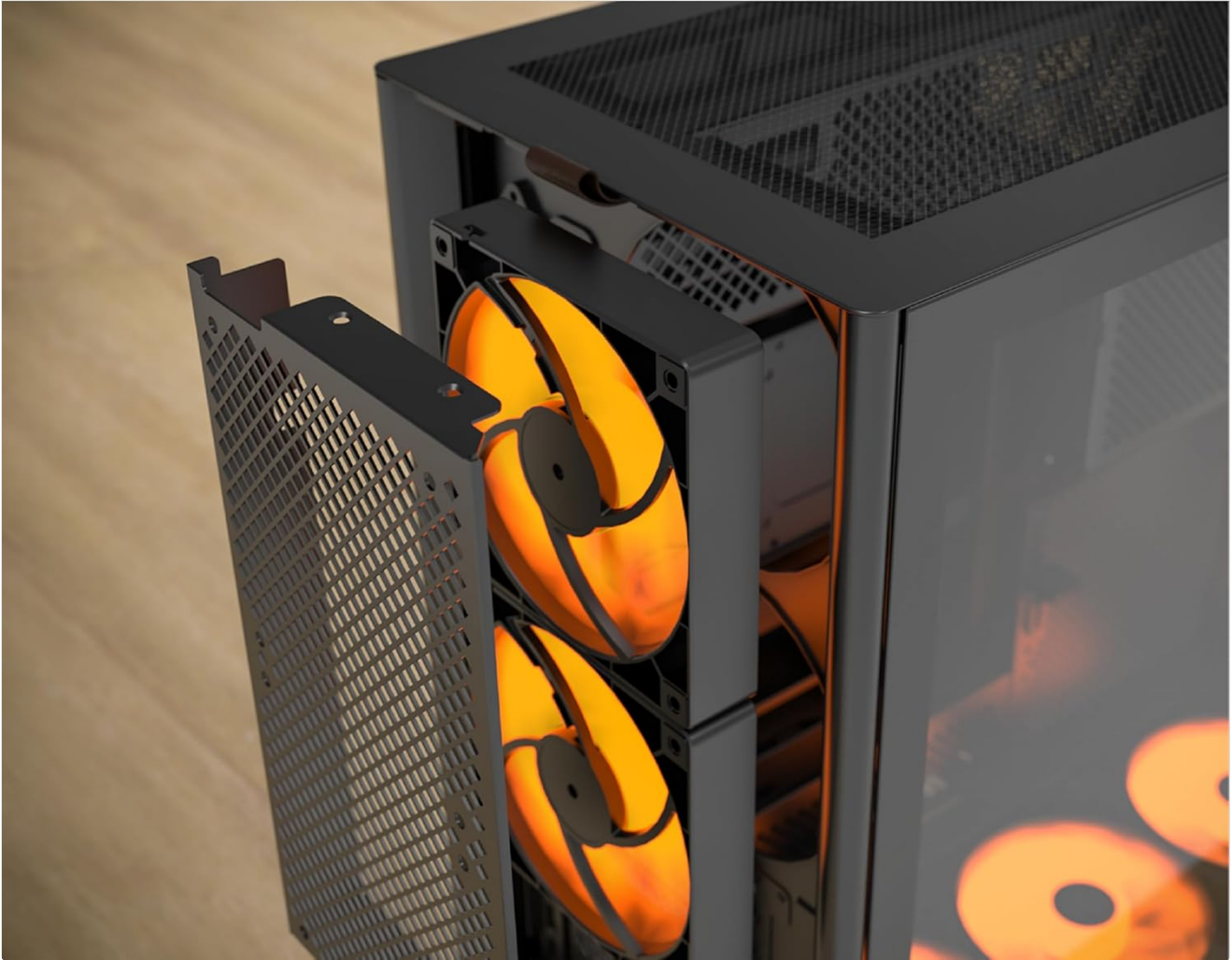
Figure 3.8: Image showing the repositioned rear fans for optimized cooling potential.
