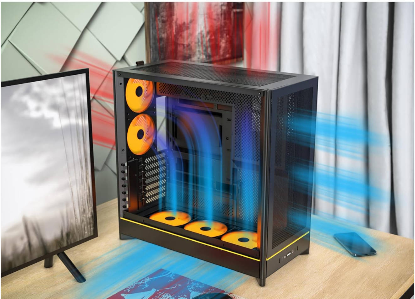
Figure 5.1: Illustration of the chimney-style cooling, showing airflow from bottom intake to top exhaust.
