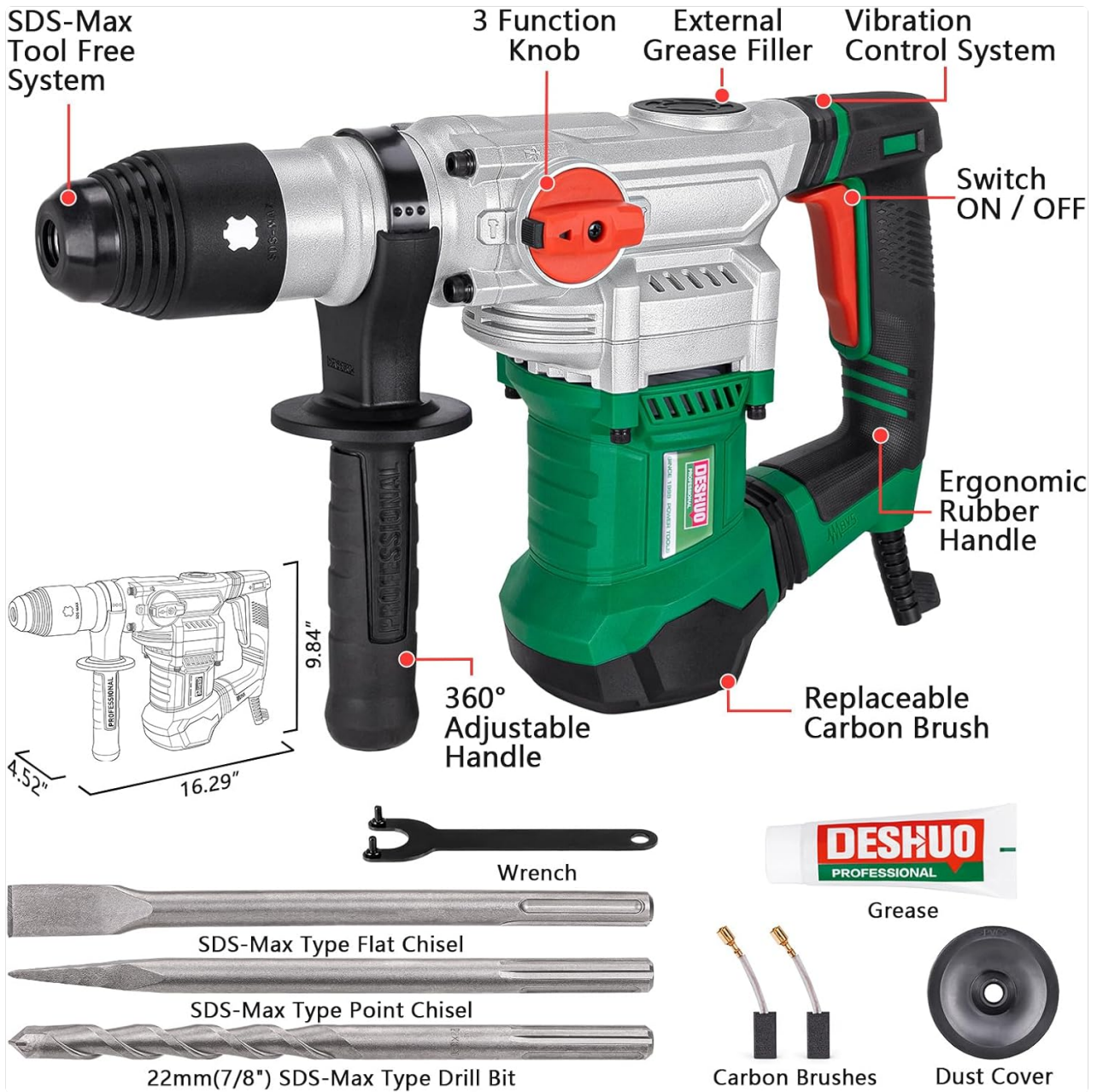
Key components of the DESHUO Rotary Hammer Drill.
