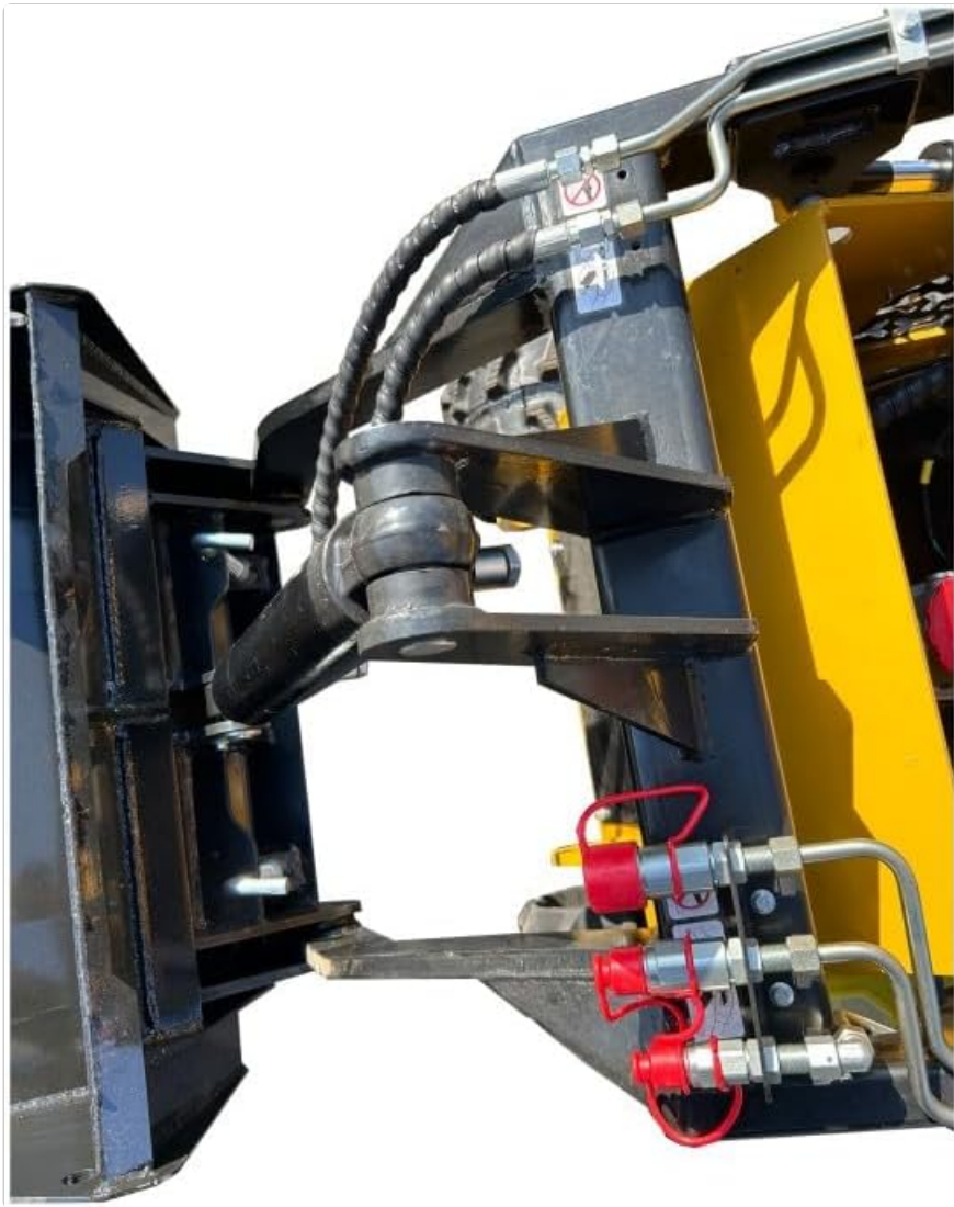
Figure 3: Close-up view of the bucket attachment points, illustrating how the bucket connects to the loader arms.
