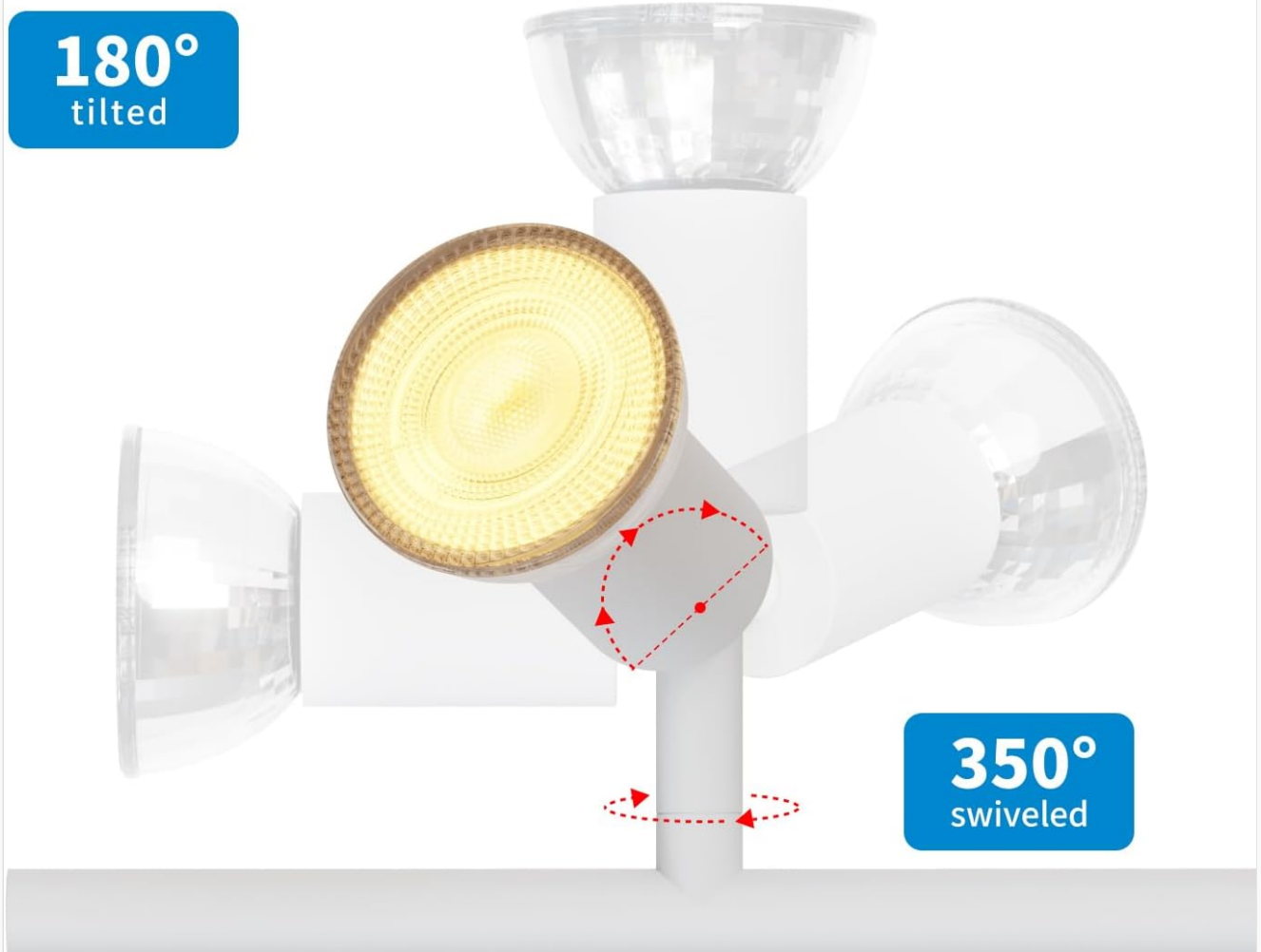
Image 6.1: Visual representation of the 180-degree tilt and 350-degree swivel capabilities of each light head.
