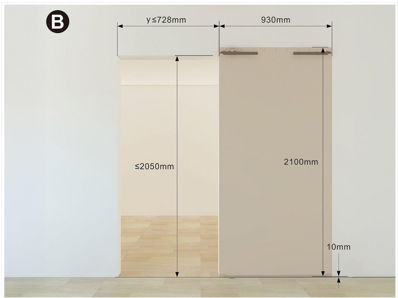
Image: Diagram B provides an alternative view of the required dimensions, reinforcing the need for adequate space for the door to slide. The door maintains a 10mm gap from the floor.
