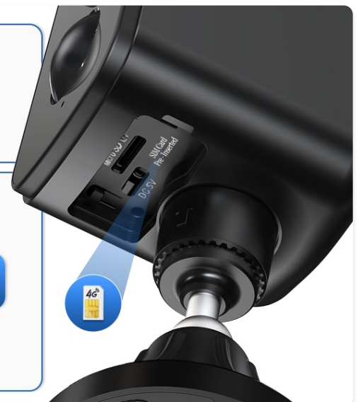
Figure 3: The camera features a pre-installed SIM card compatible with major US carriers. An SD card is not included.
