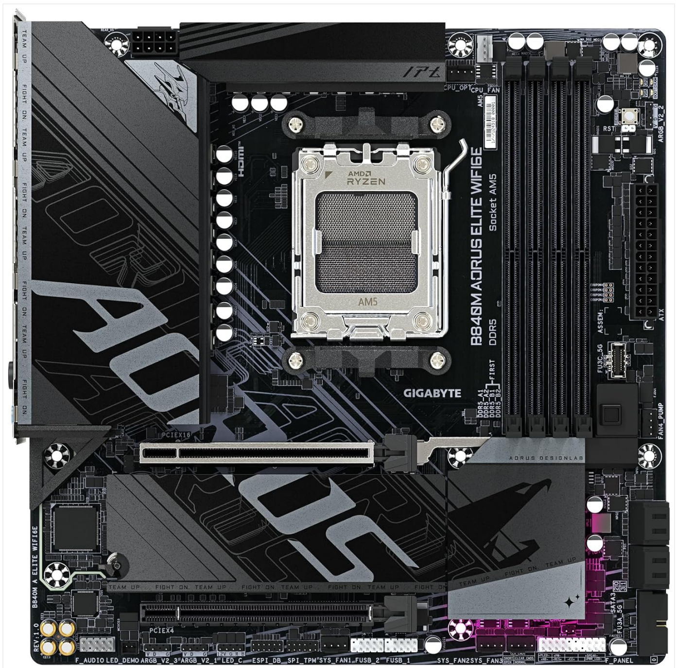
Figure 2: A top-down perspective of the GIGABYTE B840M AORUS ELITE WIFI6E Motherboard, highlighting the CPU socket (AM5), DDR5 DIMM slots, PCIe slots, and M.2 slots. This view is useful for identifying component placement.
