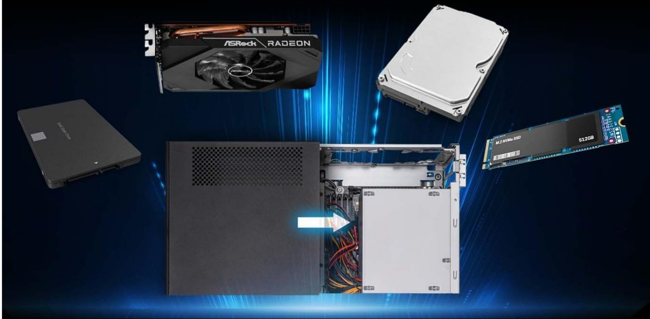
Image: Diagram showing the drawer-style chassis design of the DeskMeet X600, allowing for easy installation and upgrade of components like graphics cards, hard drives, and M.2 SSDs.
