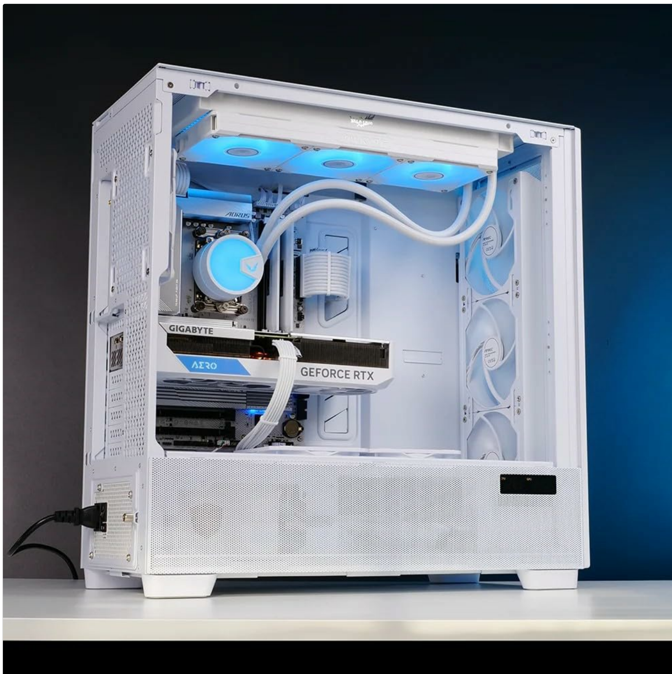
Image: The Valkyrie A360 AIO cooler fully installed within a white PC case, showcasing the blue ARGB lighting on the fans and CPU block.
