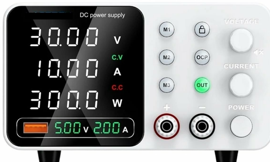
Figure 1: Front panel of the Bolisila TPS-C3010 DC Power Supply.
