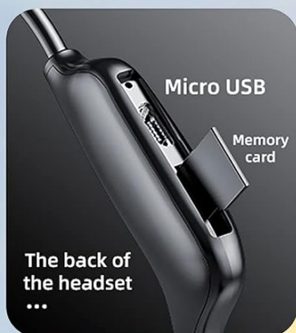
Figure 4.1: BL13 Headphones in use, illustrating key features and the Micro USB charging port/memory card slot. The design emphasizes ergonomic fit, stable balance, and unlimited movement. Features include Acoustic Conduction Technology, Waterproof and Sweatproof design, Lightweight and Portable build, Bending without deformation, Extended Battery Life, Dynamic Sound, and HD Call capability.
