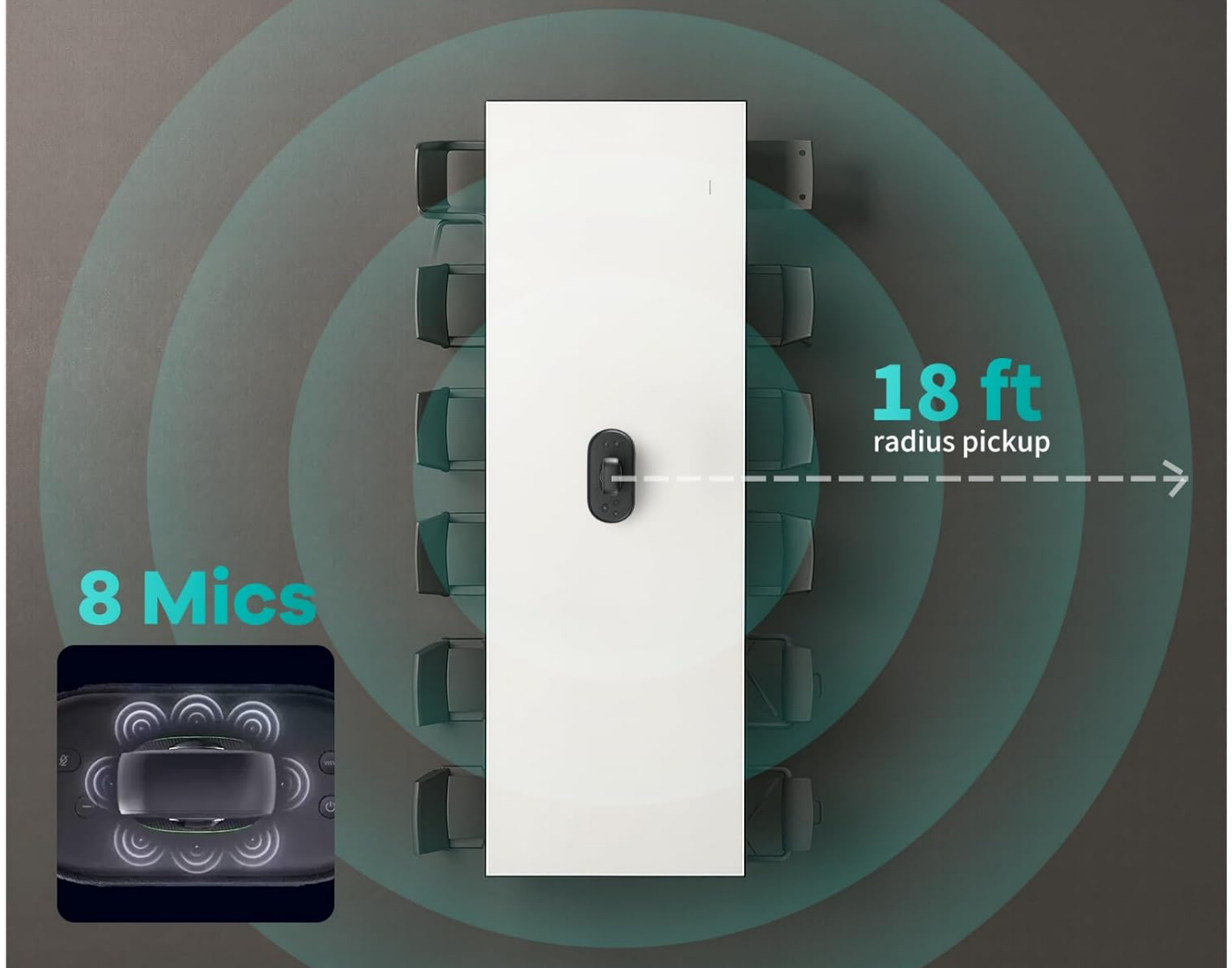
Figure 5: Diagram showing the 8 omnidirectional microphone array and its 18 ft (5.5 m) radius sound pickup capability.
