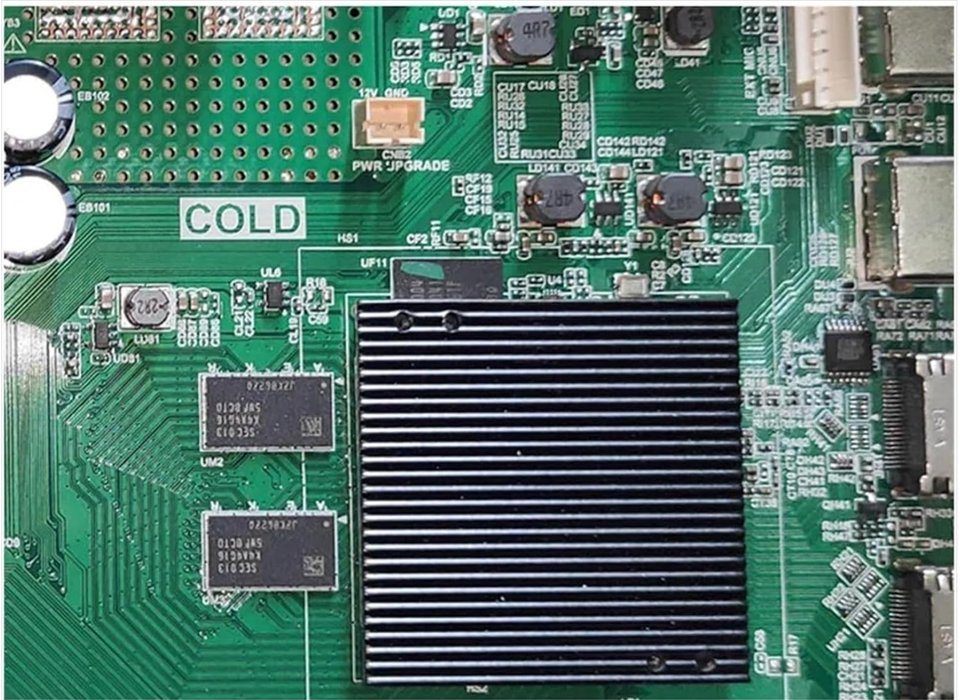
Figure 5.1: Close-up of the heatsink and memory components on the motherboard, highlighting areas critical for thermal management.
