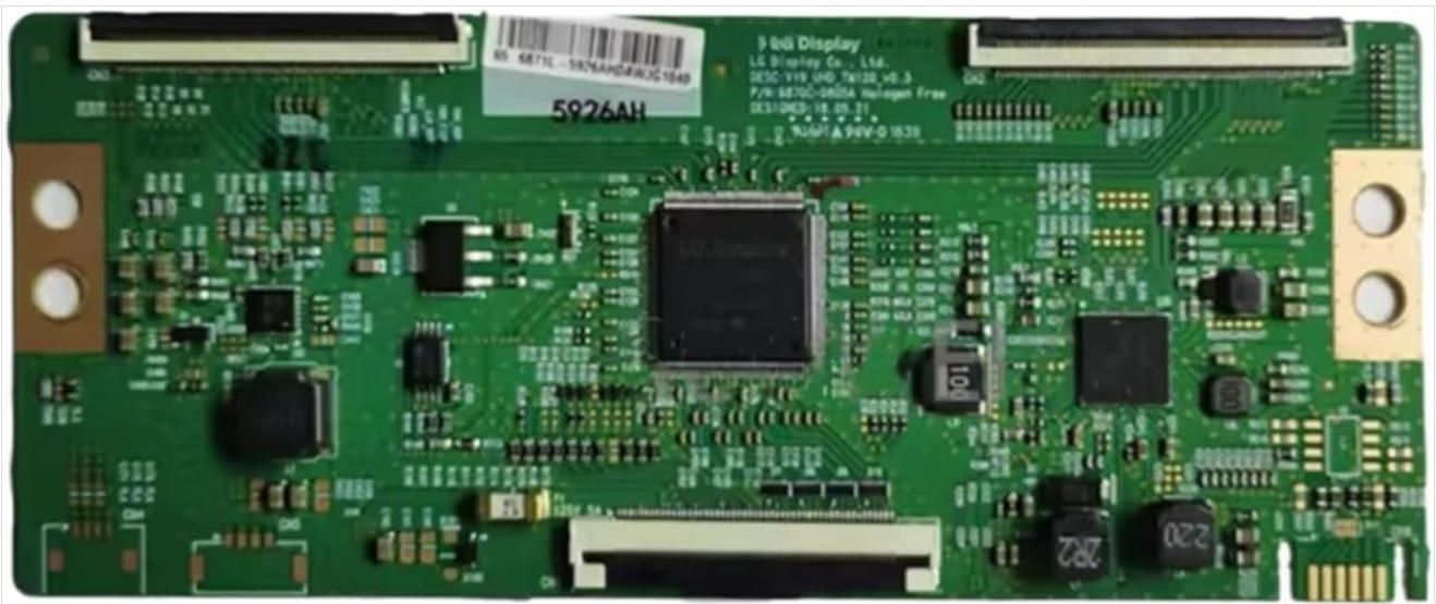
Figure 2.1: Top view of the Xqscvqwa 6870C-0805A TCON Board, showing the main chip and various components. This image provides a clear view of the board's layout and primary integrated circuits.
