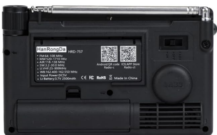
Figure 2.5: Rear view of the HRD-757 radio, displaying the battery compartment cover,
