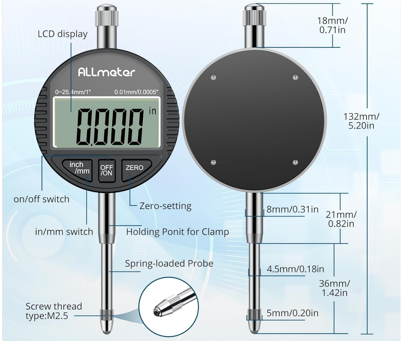
Figure 2: Detailed diagram illustrating the key components and dimensions of the digital dial indicator, including the LCD display, on/off switch, inch/mm switch, zero-setting button, holding point for clamp, spring-loaded probe, and screw thread type M2.5.
